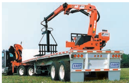
Built-in traveling unloading crane
