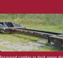
Increased camber as deck opens due to extensive deck length, offering greater hauling capabilities.
