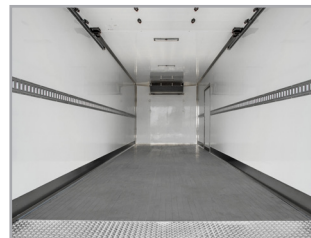
Composite floor system and seamless sidewall construction
