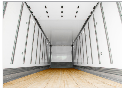
Fork truck capable floor system Bonded DuraPlate nose and sidewalls
